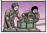
BEFORE LAUNCHING, WE GOTTA **REMOVE** THE TAIL HOOK PIN, TOO. THAT LOWERS THE TAIL HOOK SO THE SHAPOW STOPS WHEN LANDING. IF WE FORGET TO TAKE OUT THE PIN, THE TAIL HOOK WON'T CATCH THE PRIMARY PENDANT DURING LANDING AND THE SHAPOW CAN **OVERSHOOT** THE RUNWAY. WE CAN'T AFFORD TO LOSE THE **ONLY** MISSION-CAPABLE CRAFT WE HAVE.
